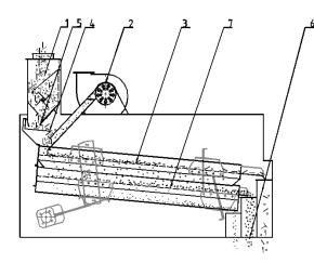
The raw material is conveyed down into the inlet bin (1). There must always be material in this bin to ensure an even distribution over the presuction area (extra equipment) (2) / top screen layer (3). The feeding device (4) doses the quantity of raw material from the inlet bin to the presuction unit / top screen box via a regulating damper.
