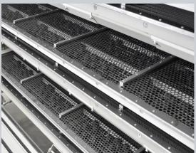
High operational reliability Perforated screens with sturdy steel frames are kept clear by a service-proven rubber ball cleaning system.
