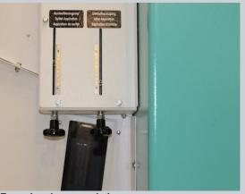
Easy air volume regulation Air volume regulation on the machine and a vertical sifter with an adjustable cross-section and inspection windows ensure optimum cleaning quality for the products.
