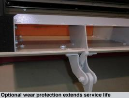
**Optional wear protection extends service life** Rhino-Hyde lining on the cleaning machine provides optimum protection against wear and noise during operation.
