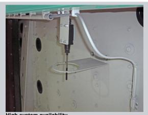
**High system availability** Safety equipment such as the oscillation monitor on the screen box provide protection against system malfunctions.
