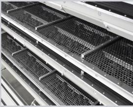
Easy maintenance thanks to access from the front to change screens For optimum accessibility the screens are changed from the
