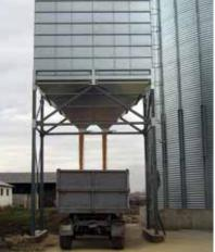
**BULK LOADING BINS** Tornum bulk loading bins are available in many different sizes and can be ada pted for a variety of loading applications.
