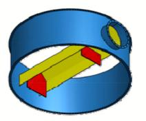
The SimPact<sup>®</sup> 4T-R construction form 17 and 17 WB have radial filter inlet with an integrated diffuser system, introducing the airflow below the filter bags.
