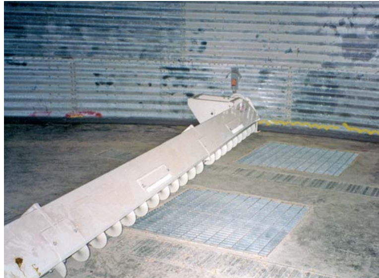
The SPIROGYRE in its parked position - close to the silo door and over the trench.
