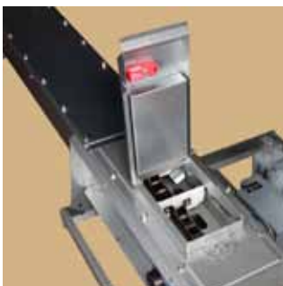
Pop up overloading flap/inspection hatch with safety switch.
