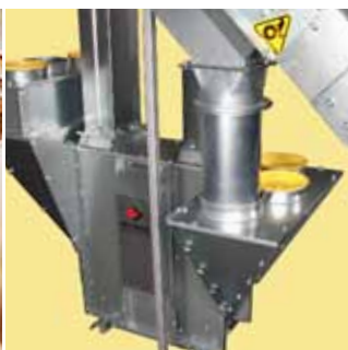
Connection to inlet hopper.
