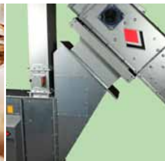
Connection hopper between conveyor and elevator.
