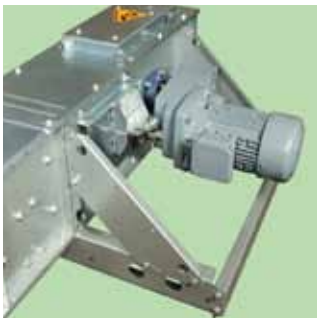
Direct-mounted gearbox motor with support frame.
