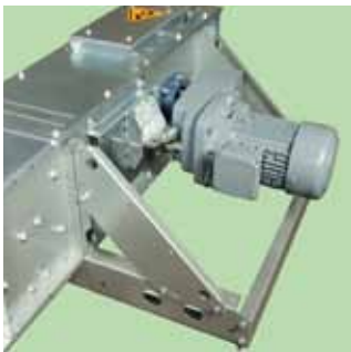
Direct-mounted gearbox motor with support frame.
