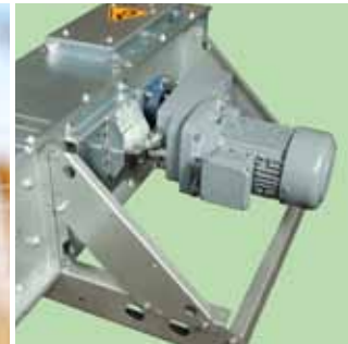
Direct-mounted gearbox motor with support frame.
