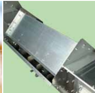
Self-regulating trench intake section.
