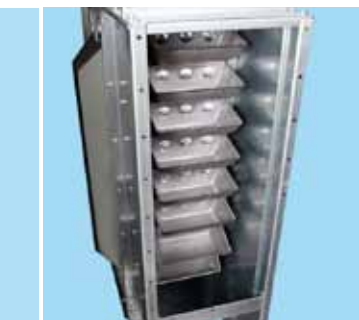
Antistatic bucket belt with steel buckets.
