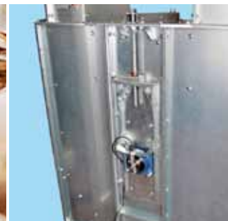
Belt tension in boot & speed monitor.
