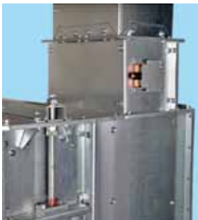
Inductive belt alignment switch.
