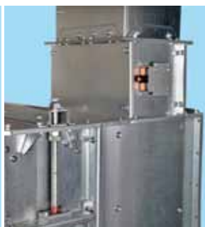
Inductive belt alignment switch.
