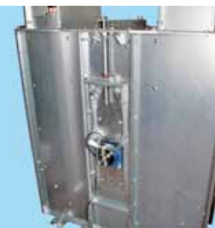
Belt tension in boot & speed monitor.
