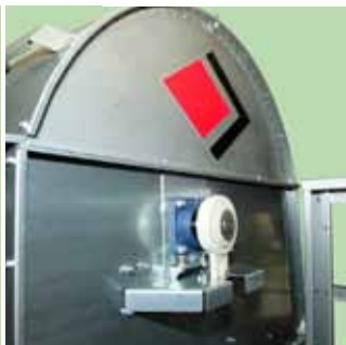
Back stop on slatted pulley in the elevator head.
