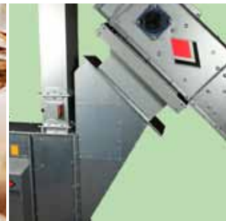
Connection hopper between conveyor and elevator.
