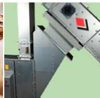
Connection hopper between conveyor and elevator.
