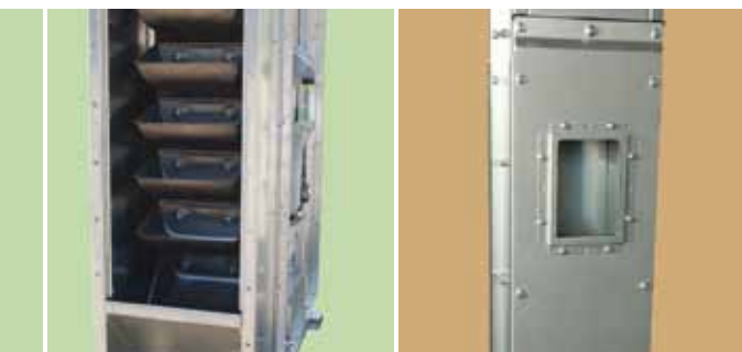
Antistatic bucket belt with steel buckets.
