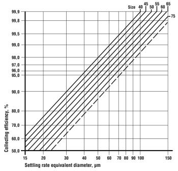
The chart above is applicable at an inlet velocity of 18 m/s and a dust concentration of 5 g/m³. At a velocity of 12 m/s, use the next line on the right. The settling rate equivalent diameter of a particle is the diameter of a sphere with a density of 1 g/cm³ which, in air at 20 °C and 1013 bar (760 mm Hg), has the same falling velocity as the relevant particle.
