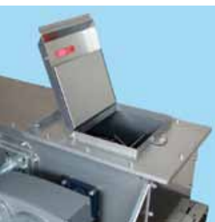
Pop up overloading flap/inspection hatch with safety switch.
