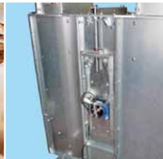
Belt tension in boot & speed monitor.
