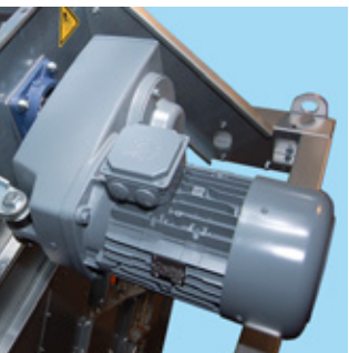
Direct-mounted gearbox motor with support frame.
